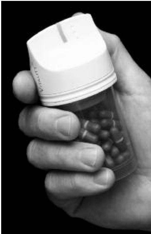
The Glowcaps product sports a digitally enhanced top that reminds a user every 24 hours to take a pill. The display automatically resets when the top is taken off the bottle. Alternatively, the user can buy a more complex version that connects to the Internet to keep track of usage.
